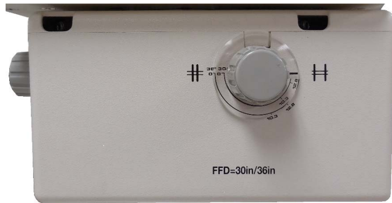
FIGURE 1.6 COLLIMATOR FRONT VIEW
